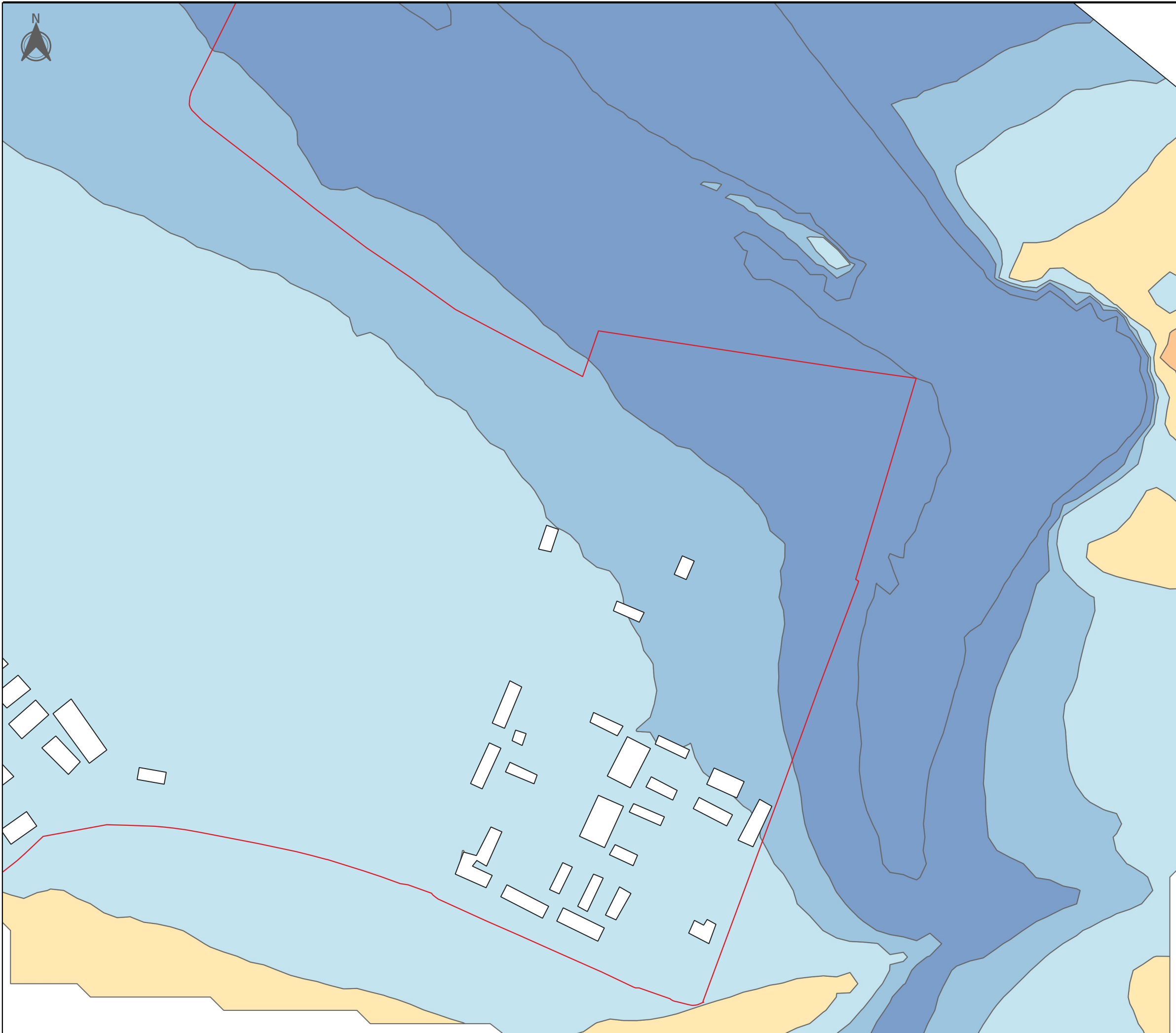
Figure 10.17 Long-term Development Generated Road Traffic Assessment without mitigation - Noise Contours 'difference contours' dB LA10,18h - Grid Height at 1.5m
